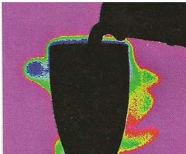
Fig 1 (a) Infrared thermography image of the gaseous CO 2 that flows out of champagne during the classic pouring method. (C&EN Chemical & Engineering News. P. 34. July 26, 2010)
